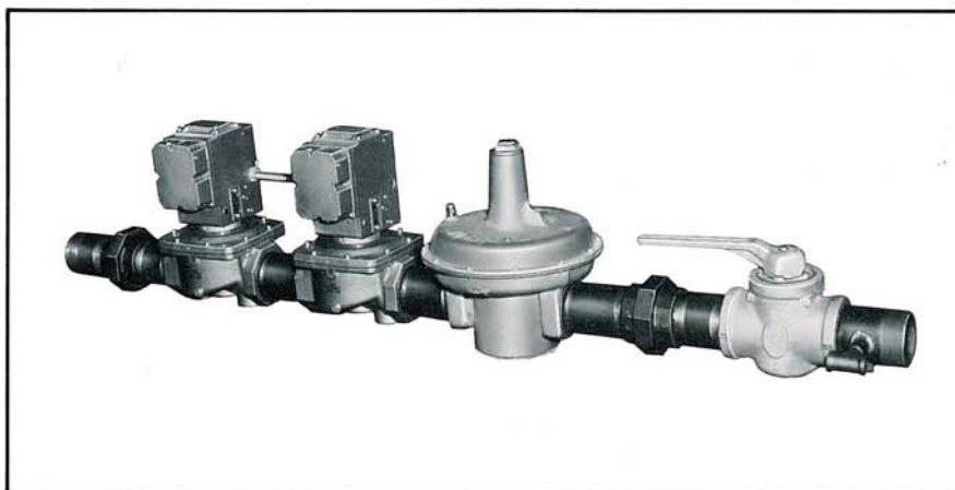
Standard Kewanee gas train with plug gas cock, gas pressure regulator, automatic gas valve, independent automatic safety gas valve (over 1 million BTU/hr.), gas volume control valve and pressure gauge. Exceeds U.L. requirement.
