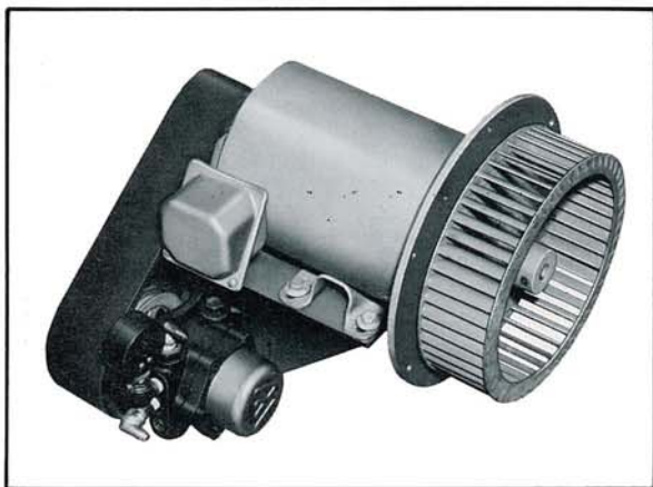
Kewanee's special power-pack, easily removable as a single unit for servicing. Front-drive fan wheel and rear-drive oil pump are driven by same motor.
